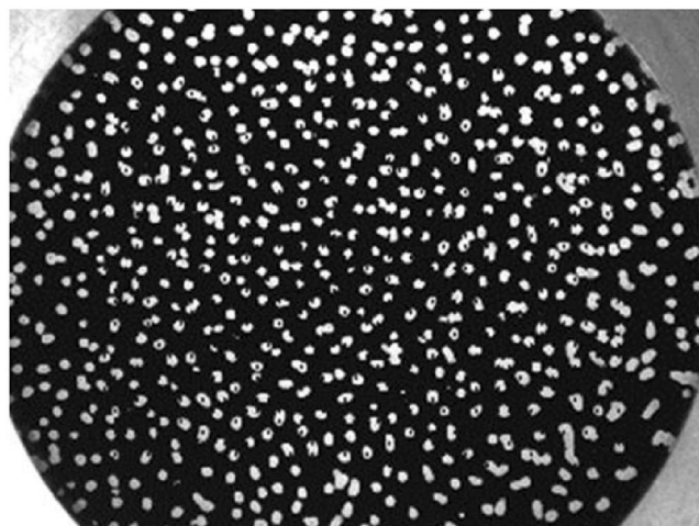
Fig. 7 Digital image of MEA coupon T1 (with white dot contrast pattern) in drum fixture. Note that portions of the digital grid superimposed on the coupon image appear as small black dots on the white dots.
