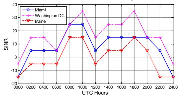
Fig. 1. Simulated SINR during the course of 24 hours in Miami, Washington DC, and Maine (provided by SPAWAR, US Navy)
