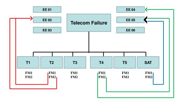
EE = End Effect FM = Failure Mode T(x) = Transformer #
