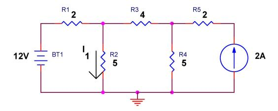
6. In the circuit below use a loop analysis to specify the voltage source  $V_S$  so that 20 watts of power are dissipated in the  $5\Omega$  resistor. Be sure to provide both solutions.
