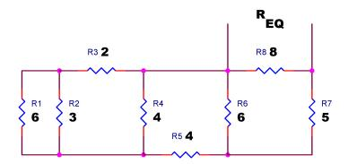
2. Find the equivalent resistance  $R_{eq}$  in the circuit below.
