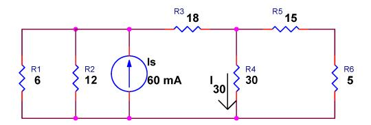
5. Use a loop analysis method to find current  $I_1$  in the circuit below. Identify all the nodal voltages in the circuit and specify their values using 3 decimal points of accuracy.
