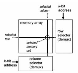
Figure 3. Nanoscale memory array using crossbar structure [18].
