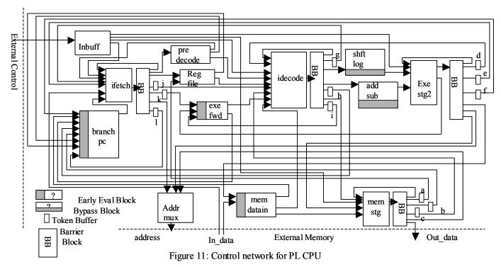
buffer adds forward latency to the path, so the extra latency must be offset by the time gained from not waiting on feedback. These buffers are placed in the netlist by the partitioner; an external data file read by the partitioner specifies buffer locations. This frees the designer from having to pollute the input VHDL netlist with buffers.
