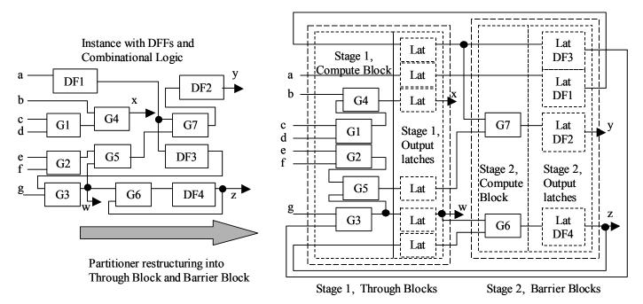
Figure 10: Restructuring of instance with DFFs/combinational gates into Through, Barrier blocks
