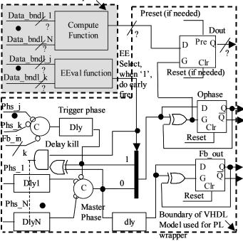
Figure 4: Coarse-grain PL block with early evaluation
