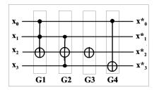
Figure 1. A cascade of 4 gates with 4 variables
