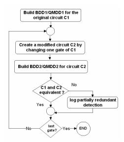
Figure 2. Detection of partially redundant logic
