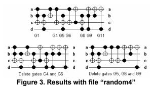
This reversible circuit (shown in Fig. 3 using Maslov's RCviewer tool [5]) of 11 gates captures hidden replacements using the exhaustive gate deletion. We found that deleting gates  $\{G4,G6\}$  or  $\{G5,G8,G9\}$  does not alter the functionality of the circuit.
