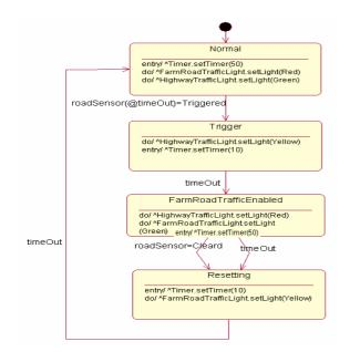
Figure 4. UML State Machine Diagram for Traffic Light Controller
