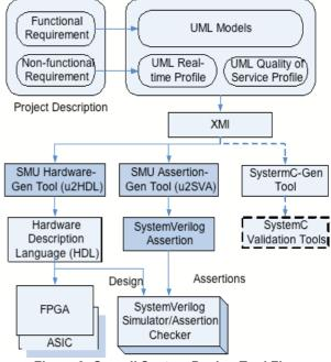
Figure 3. Overall System Design Tool Flow
