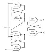
Figure 6. Diagram of D-flip-flop using MIN-inversion Gates
