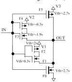
Figure 2. Quaternary Inverter Circuit
