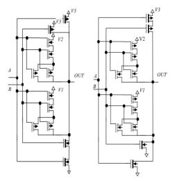
Figure 5. MIN-inversion and MAX-inversion Circuits
