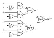
Figure 7. Diagram of 4:1 Mulitplexer
