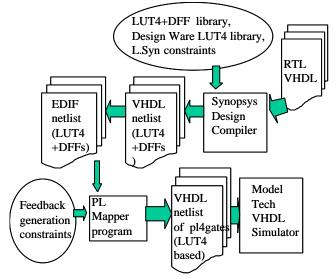
Figure 8: Clocked netlist to PL netlist methodology
