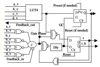
Figure 3: LUT-4 Based Phased Logic Gate
