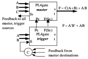
Figure 4: An Evaluation Gate from Two PL Gates
