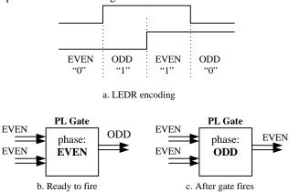
Figure 1. LEDR Encoding and PL Gate Firing
