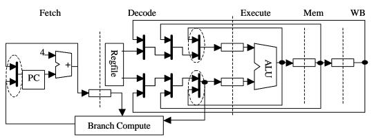
Figure 7: Simplified CPU Datapath Diagram
