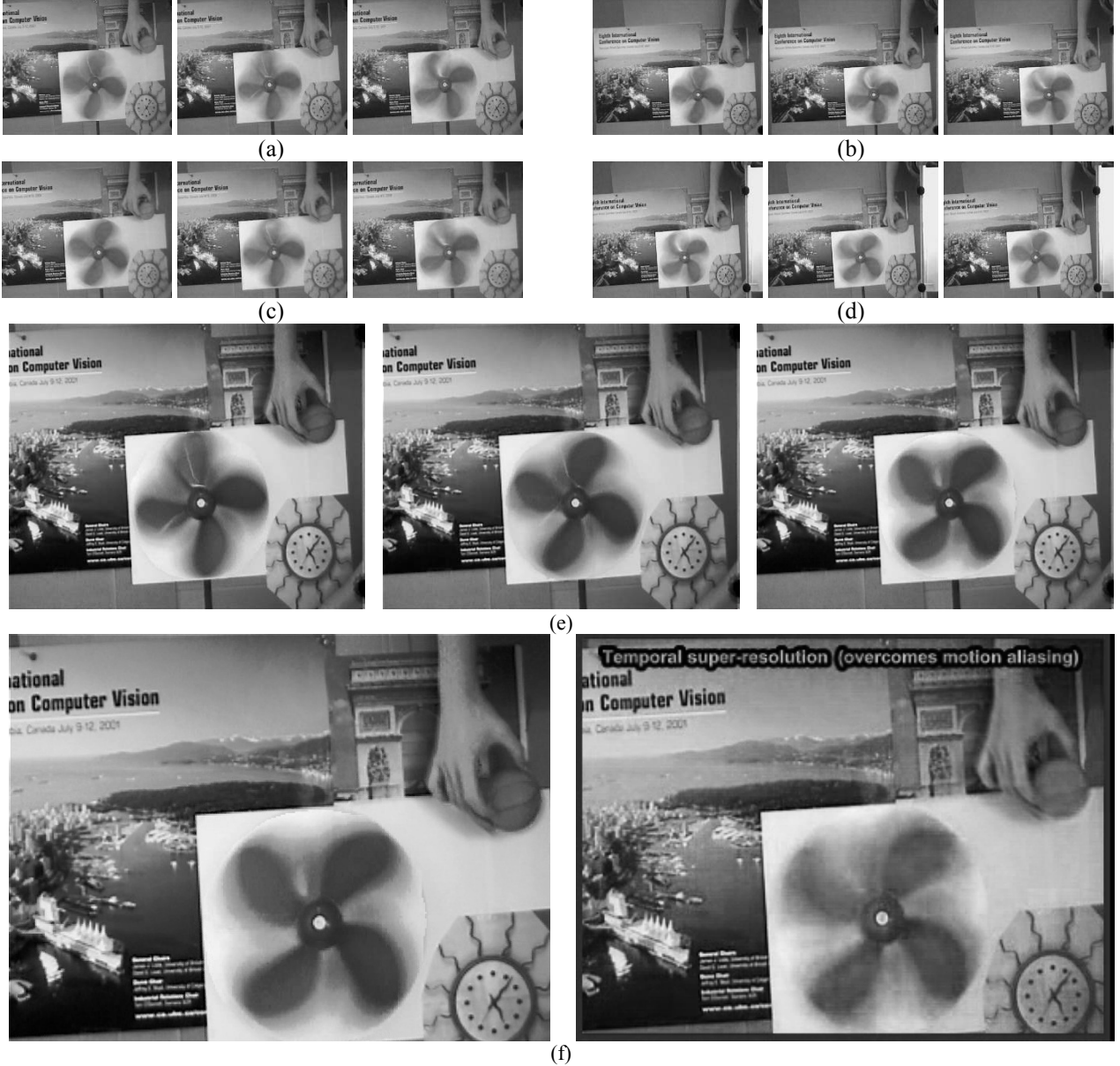
Fig. 2. The “wagon wheel effect” appeared as a result of motion aliasing. (a)-(d) Three successive frames from one of four PAL video recordings of a fan rotating clockwise. The fan seems to be moving counter-clockwise. (e) Six successive (left to right, up to down) frames of the reconstructed video in which the spatial and temporal resolutions were increased by factors of 2 and 3, respectively. Now the fan is rotating in the true direction. (f) Comparison between a reconstructed frame with the proposed method (left) and with the result reported in [3] (right; converted to gray-scale).
