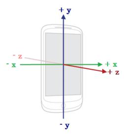
Figure 4.6. Accelerometer Device With X, Y, and Z Dimensions Grenga  $\left(2014\right)$
