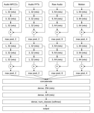
Fig. 1. Convolutional network architectures used for keystroke classification.
