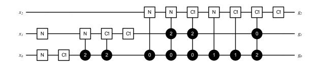
Figure 3.8: Discrete Logarithm for Three Digit Ternary Logic Designed with Automated Method
