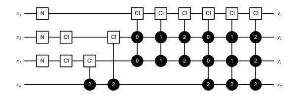
Figure 3.5: Multiplicative Inverse Circuit Design for Four Digit Ternary Logic
