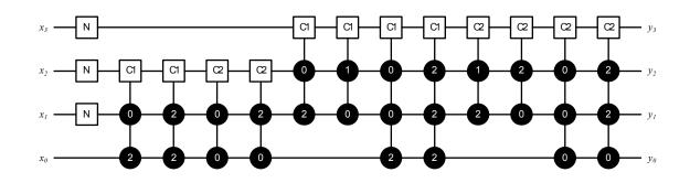
Figure 3.6: Multiplicative Inverse Circuit for Four Digit Ternary Logic with Balanced
