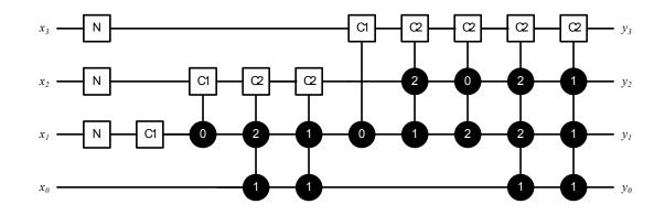
Figure 3.4: Final Multiplicative Inverse Circuit Design for Four Digit Ternary with Modular Digit Value Encoding
