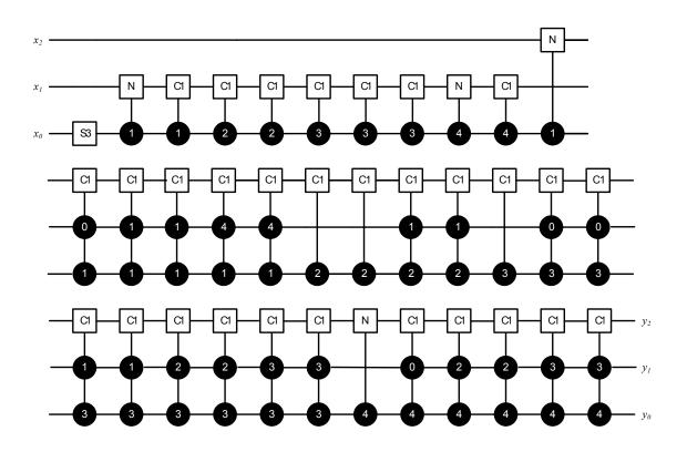
Figure 3.14: Multiplicative Inverse Circuit Modulo 5<sup>3</sup> with Negative Modulo Equivalent Encoding
