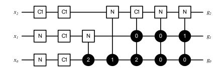
Figure 3.7: Discrete Logarithm for Three Digit Ternary Logic
